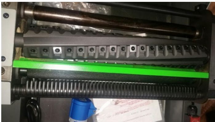
Helical cutter block significantly reduces noise level in classrooms
